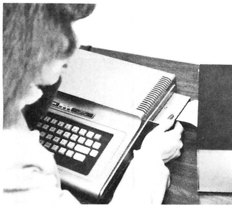
1. Here is Jeri plugging The Solution into the CoCo. Then she will move the main case up close to the CoCo. The cable is kept short to prevent noise and interference. The disk controller can be plugged into the side slot. The power supply plugs into a socket on the back of the case. All wires for the internal boards exit out the back of the case.
